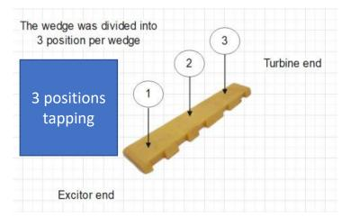
Slots were numbered starting at slot number 1 at NDE. Each wedge was tapped three location (3 times tapping) at the middle, and once each side of middle, recording the individual values then average of the three values.
